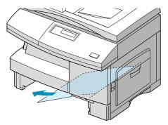
Once you remove the jammed paper here, open the side cover and then close it to clear the "PAPER JAM" message on the display.
